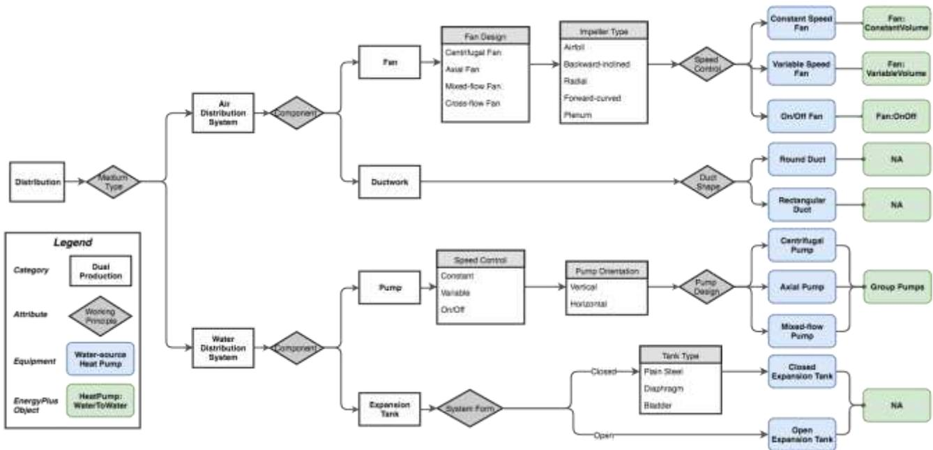
Figure 2 Classification map of heating and cooling medium distribution components.
